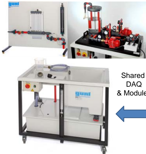
Interchangeable experiment modules for demo of fluid flow principles
